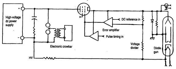
Figure 16-4. Modulator switch and regulator series tube in positive return of high-voltage power supply.
