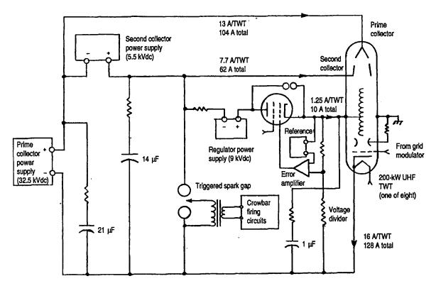
Figure 16-3. Electronic linear voltage regulator that handles only TWT body current.
