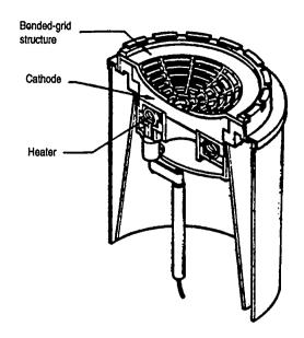
Figure 8-5. Cross-section view of electron gun with control and shadow grids.
