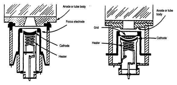
Figure 8-3. Cross-section view of electron gun with insulated focus electrode.
