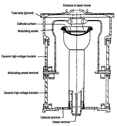
Figure 8-2. High-power microwave-tube electron gun with modulating anode.
